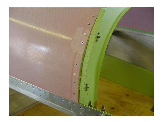
Install the F-1007CT and F-1008CT bulkheads using AN470 4-3 rivets.
