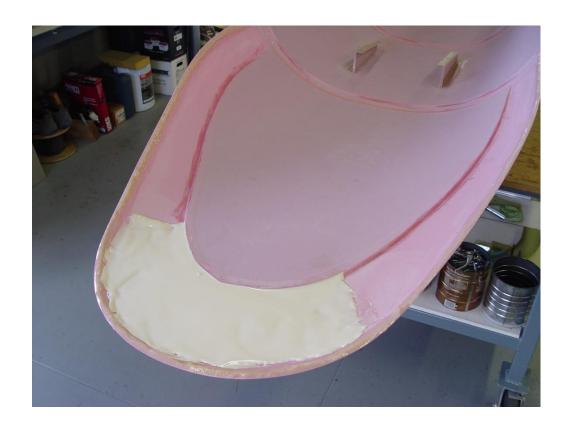
Carefully install the skin and cleco in location, clean off excess epoxy as needed. After the adhesive has cured rivet the skin to bulkheads starting at the top working down each side. Rivet the splice plate to the skin and backing plate starting at the midpoint working fwd then aft, use CS4-4 blind rivets for attachment.
