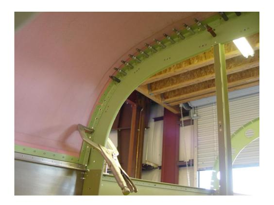
Reinstall the F-1006CT-L&R bulkheads, rivet using AN4264-3 and AN4704-3 rivets, you may want to leave the F-1028 vertical reinforcement out until you no longer need access into the tailcone. Reinstall the F-1006ECT angle and rivet to the bulkheads using AN4263-3.5 rivets. Use CS4-4 rivets in the cabin top countersunk holes and LP4-3 all other locations.
